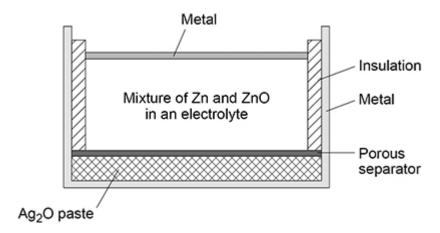
(b) Suggest the function of the porous separator in above diagram.
